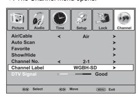
4 Press ▲ or ▼ to highlight Channel Label, then press ► or ENTER. The channel label screen opens.
